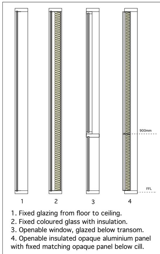
Diagram 6. Four conditions for facade glazing system.
