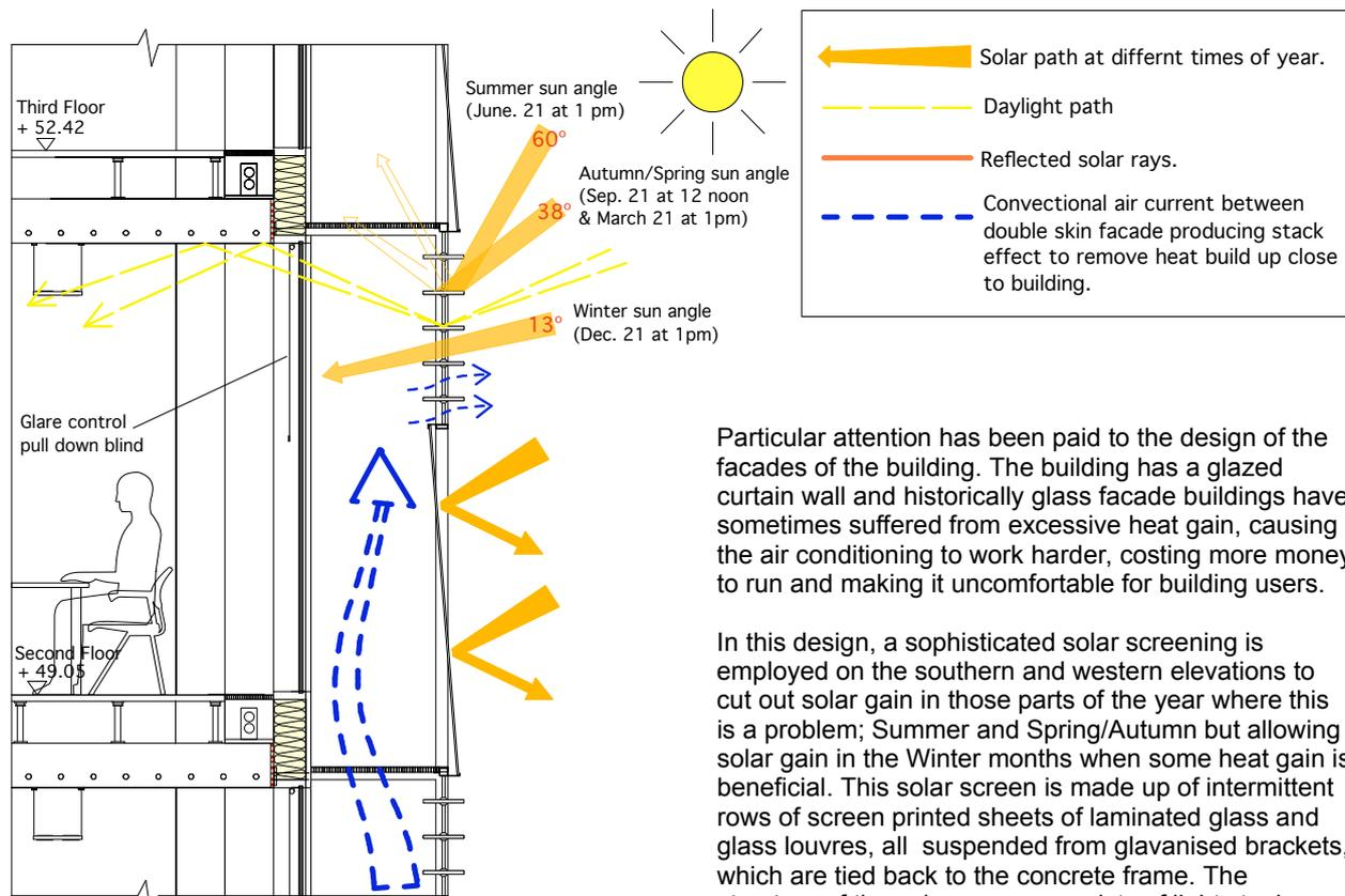
Diagram 5. Section through facade showing solar screening cutting out unwanted Summer and Spring/Autumn solar gain but allowing beneficial solar gain in Winter through the glass blades.
