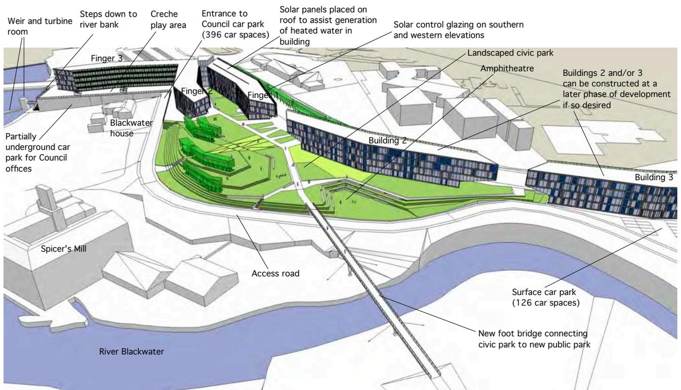
Diagram 1. Aerial view of scheme from North West showing Councils' building and buildings 2 & 3 constructed.
