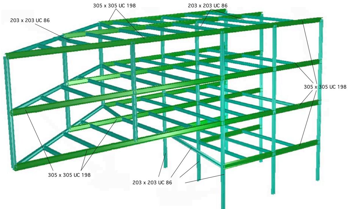
Diagram 5. Structural design for Vierendeel truss for cantilevered end sections of fingers 1 and 2.
